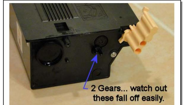
**Photo #3: Location of Extra Pair of Gears found on all 4250/4260 cartridges... Only found on some of the earlier 4150's.**
