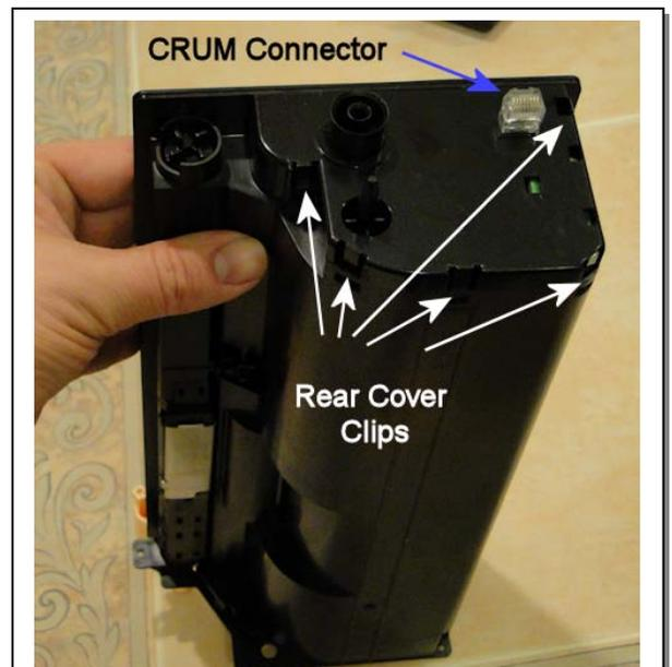
**Photo #4 & 5: Removing the Rear Cover...**
