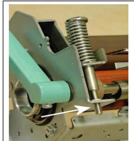
**Photo 15: Note how much of the Pressure Screws are below the frame by marking or counting threads.**
