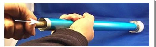
Photo #9: Use a shaft to knock the gear end off.
