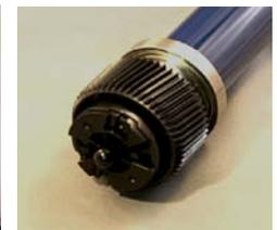
Photo #'s 10, 11 & 12: Assembling the hubs and gear.
