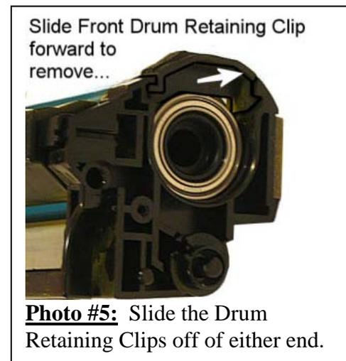
**Photo #5:** Slide the Drum Retaining Clips off of either end.
