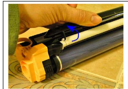
**Photo #3:** If your cartridge is the newer kind (anything but the DC250 version), first remove the cleaning roll cover by pivoting up to the left as shown.
