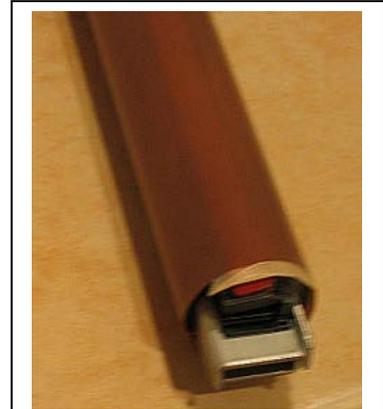
Photo 8: **End of Pressure Belt Assembly...**
