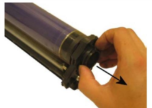
Photo #8: **Rear Drum Bushing removal.**
