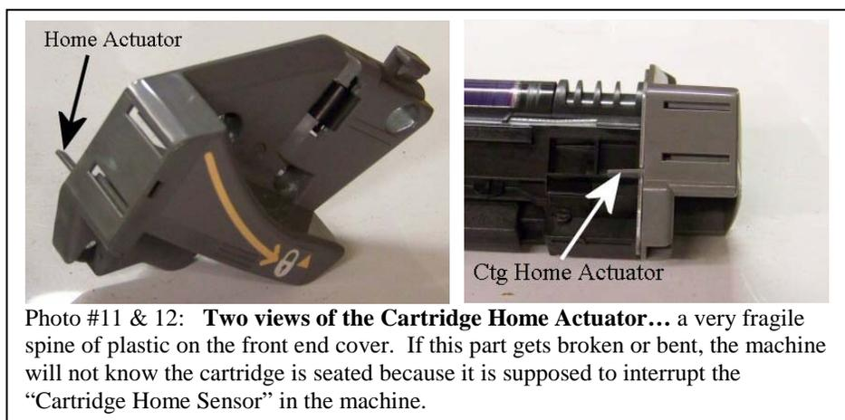
Photo #11 & 12: **Two views of the Cartridge Home Actuator...** a very fragile spine of plastic on the front end cover. If this part gets broken or bent, the machine will not know the cartridge is seated because it is supposed to interrupt the "Cartridge Home Sensor" in the machine.
