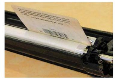
**Photo #10:** Plastic shims can be used to set the space between the Mag-Roll and Trimmer-Bar
