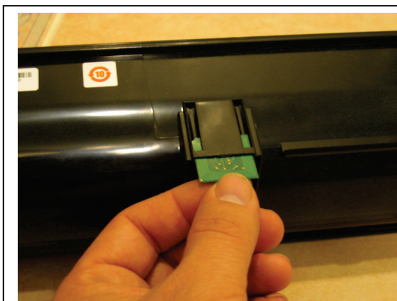
Photo # 2: Removing the Connector
