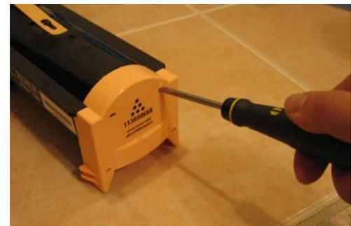
**Photo #1: Removing Front End Cover**
