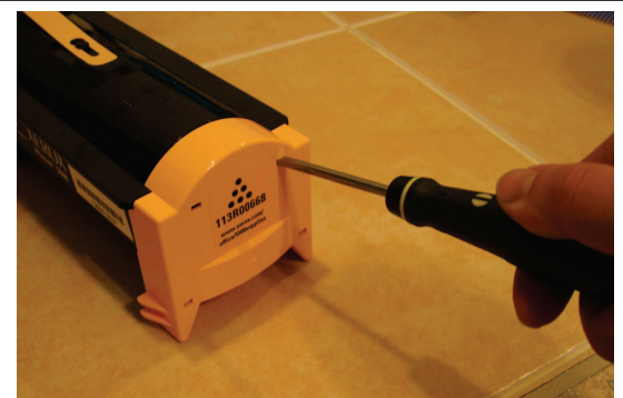
Photo #1: Removing the Front End Cap
