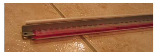
Photo #8: Drum Blade shown with the Saw Toothed mylar piece.
