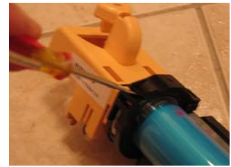
Photo #5: Releasing the front Bearing Retaining Clip...
