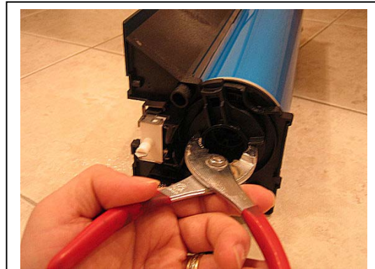
Rear Drum Hub Removal (shown with hub in removal position)
