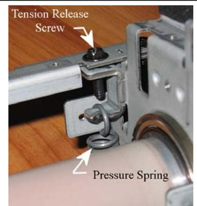
Releasing the tension on the Pressure Roller.
