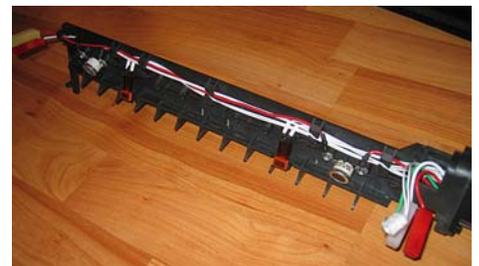
The Thermistor / Thermal Fuse Assembly.
