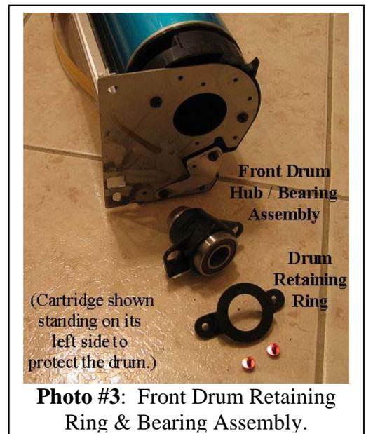
**Photo #3: Front Drum Retaining Ring & Bearing Assembly.**
