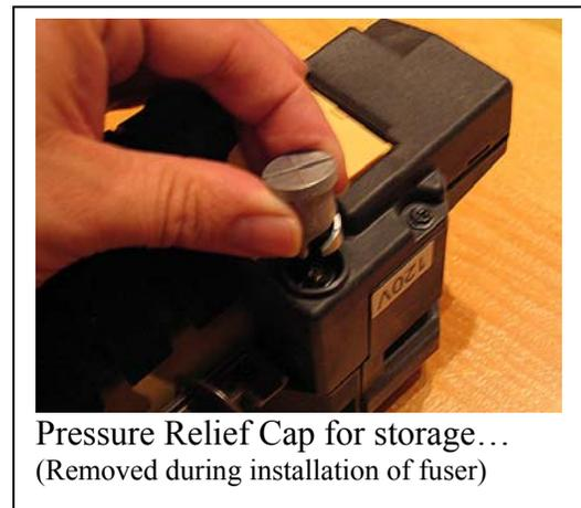
When you respond to a Fuser Related call, you'll want to bring a new fuser (or one you rebuilt earlier), and a little bit of information. First thing to do is to check out the fuser's fuser lamp circuits and the thermistor circuit as well. It'll be handy to know which pins are which on the fuser module so that you can diagnose the problem without needing to take the fuser apart.
