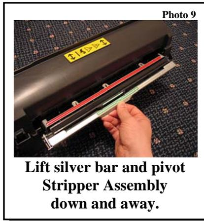
**Lift silver bar and pivot Stripper Assembly down and away.**
