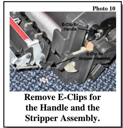
**Remove E-Clips for the Handle and the Stripper Assembly.**
