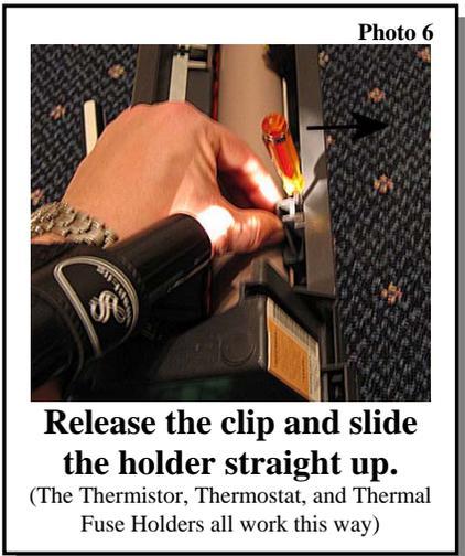
check and clean the face of the thermistor and the thermostat (see Photo 7). There is also an AC overheating fuse in the Fuser Lamp circuit which can be accessed in the same way.
