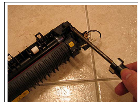
Photo #3: Removing one of the two screws which hold the two halves of the fuser together.
