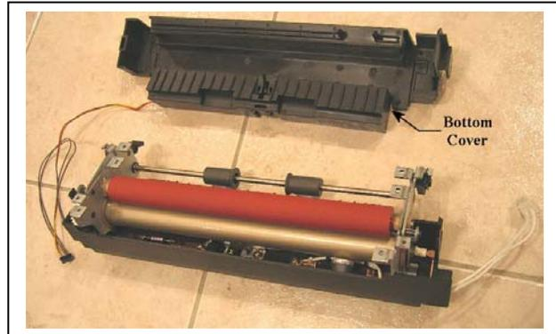
2.) Release the Fuser Lamp Rear Terminal's screw to disengage the rear terminal. You can slide the Fuser Heat Lamp out through the front end (the end opposite the gears).
