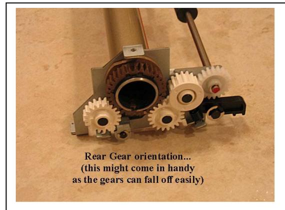
4.) To remove the Heat Roller, remove the front snap ring (opposite the gear end). Then hold the heat roll bearings in place in the metal front and rear frames, slide the roller out of the rear (geared) end. Keeping the bearing / sleeve in place will protect the heat roll from scratching against the metal frame.
